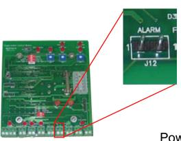
**Safety Alarm:** If the gate hits an obstruction twice while closing or opening, the system will shut down for 5 minutes. On the Board, you have two options of reset mode.
