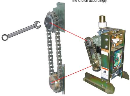
Use an appropriate wrench to adjust the clutch
