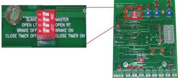
**Switch #1** must be set to the Slave or to the "off" position.
