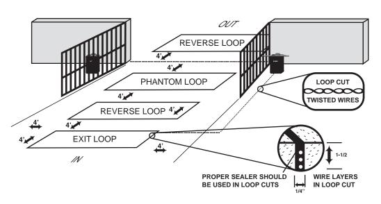
Wires must be wrapped inside the groove three times. Once you have completed the process, fill up the grooves with a proper sealant.
